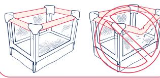
**5** Push down on center of Playard/Crib floor until it is flat and *locks* into position.
